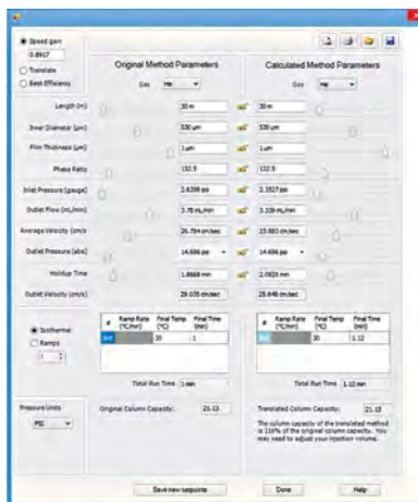
Method Calculator makes it easy to set up a method that shortens analysis time or facilitates the changing of carrier gas.
