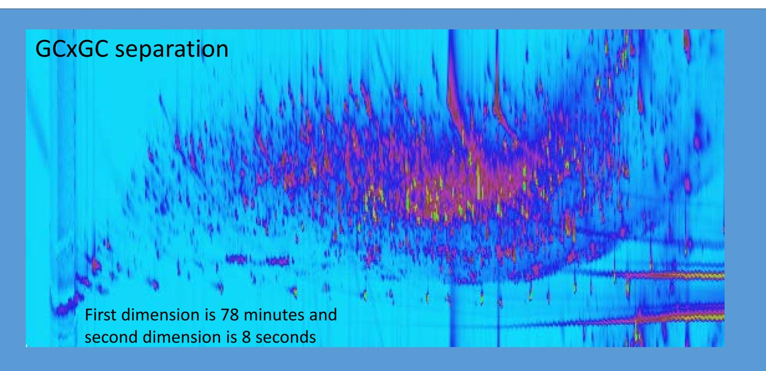
The increased peak capacity in GCxGC results in fewer co-eluting peaks, as can be seen in the analysis of a wastewater sample spiked with 30 analytes above.
